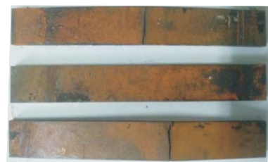
(c) 焊缝加载率 66\% \sigma_s
