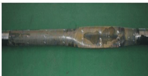
图11 套管外压挤毁后实物形貌
